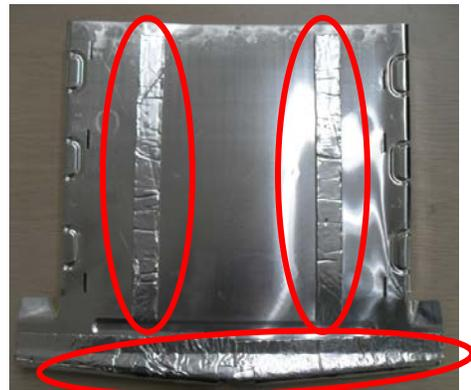
7. Bend the bottom row of the cooling ribs on the evaporator.
